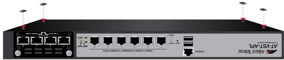
Figure 10. Attaching the Rubber Feet
