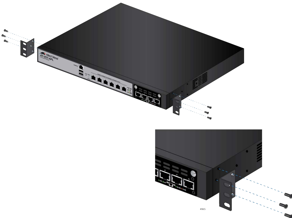
Figure 11. Attaching Brackets to the Vista Manager Appliance
