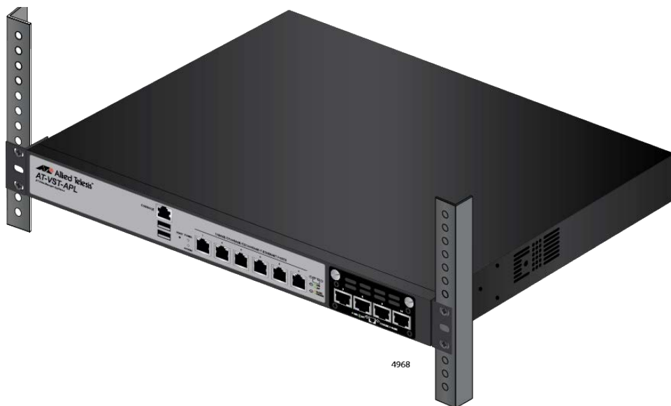
Figure 12. Mounting the Vista Manager Appliance in an Equipment Rack
