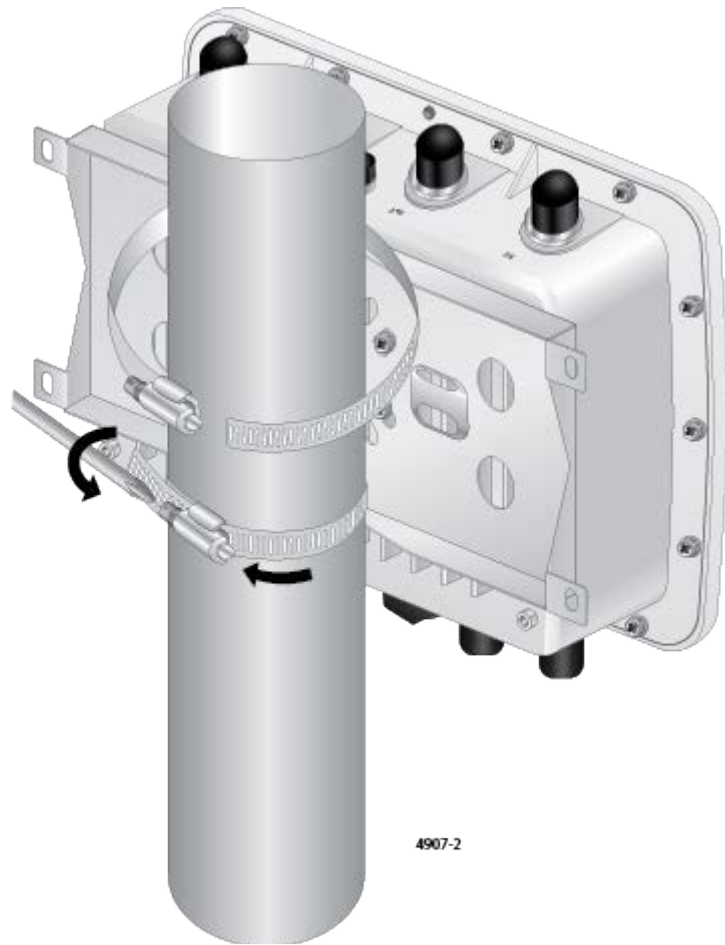
Figure 37. Tightening the Straps
