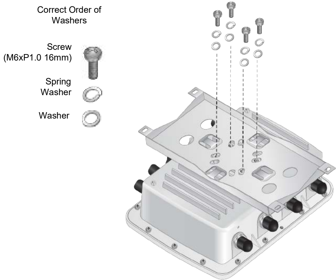
Figure 28. Attaching the Mounting Base to the Access Point
