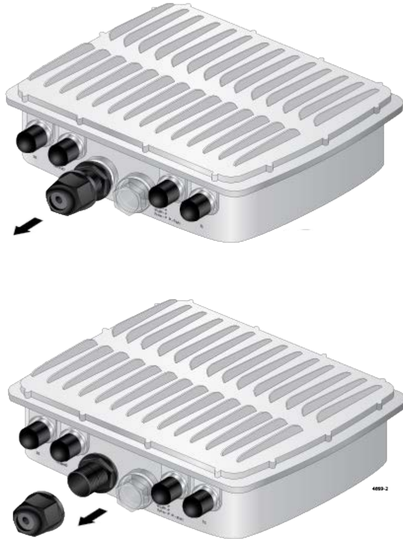
Figure 11. Removing the Cap from the LAN Port
