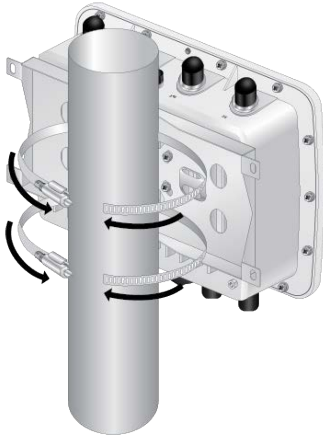
Figure 35. Wrapping the Pole Straps Around the Pole
