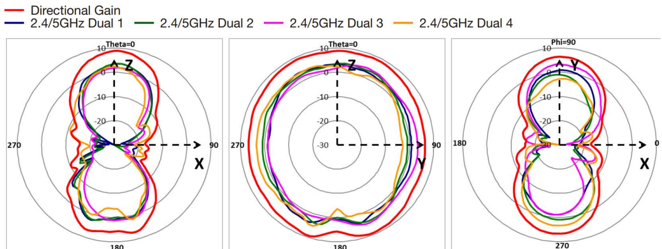
Figure 48. 2.4/5GHz Dual (2.4GHz) Radiation Patterns
