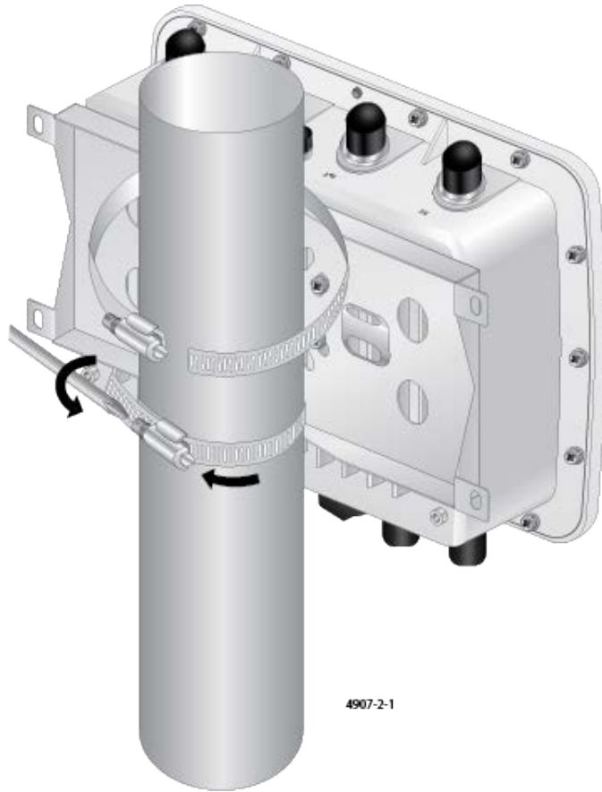
Figure 36. Inserting the Strap Ends into the Screws
