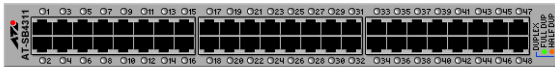
48-Port (RJ-45) 10BASE-T/100BASE-TX Fast Ethernet Line Card
