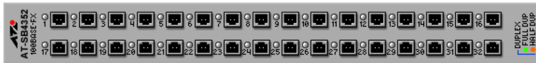
32-Port (MT-RJ) 100BASE-FX Fast Ethernet Line Card
