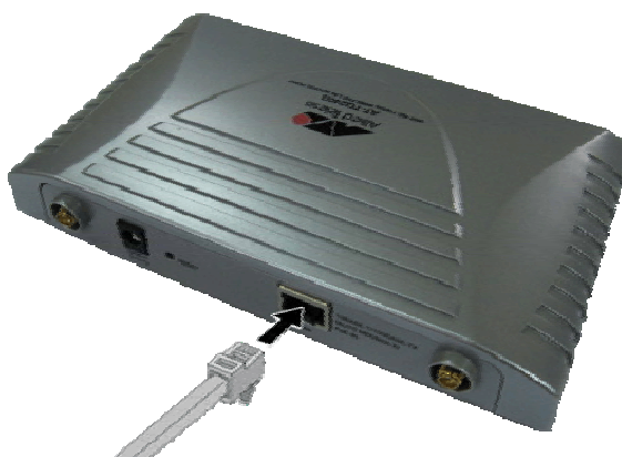
Figure 7: Attaching the LAN Cable
