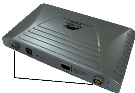
Figure 2: Location of the Antenna Connectors
