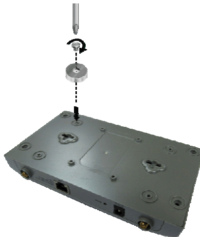
Figure 6: Attaching the Magnets
