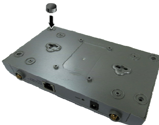
Figure 4: Attaching the Rubber Feet
