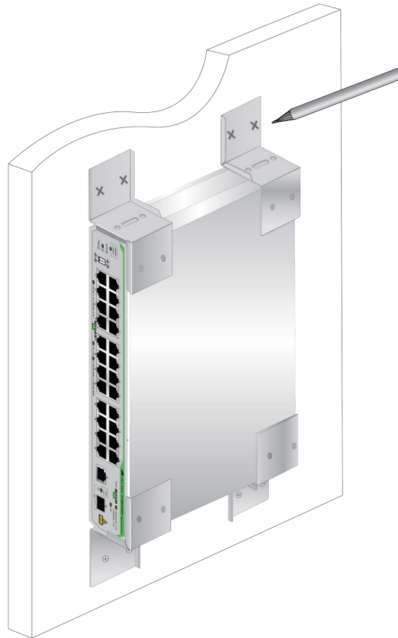
Figure 7. Marking the Screw Hole Locations for the Top Brackets
