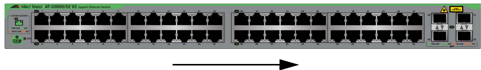
Figure 26. Ventilation Airflow of Switches with Fans
