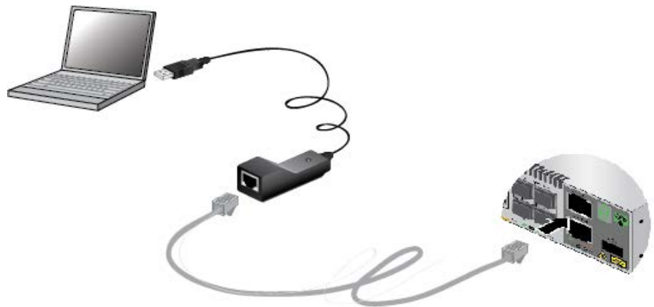
Figure 60. Local Management Session of the Switch with the VT-Kit3 Management Cable
