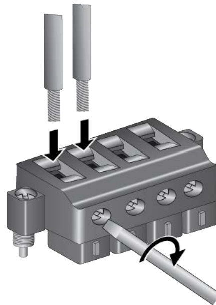
Figure 67. Inserting DC Wires into the POWER Plug
