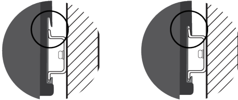
Figure 29. Installing the Switch on a DIN Rail - 3
