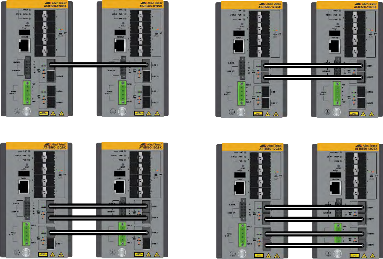
Figure 76. Trunk Examples for Stacks of Two IE560-12GSX Switches
