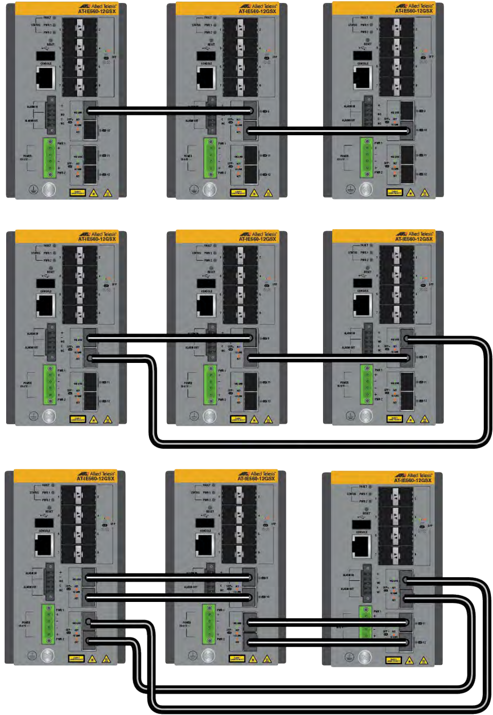
Figure 77. Trunk Examples for Stacks of Three Switches
