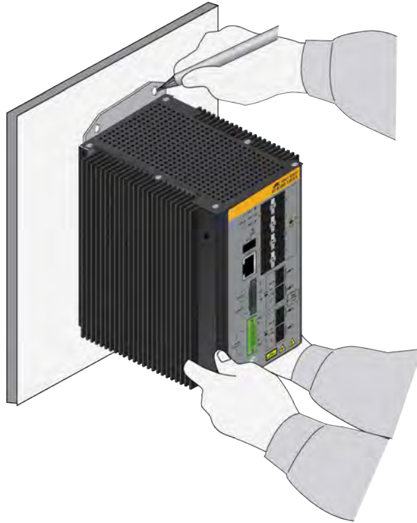
Figure 35. Marking the Bracket Hole Locations on a Concrete Wall
