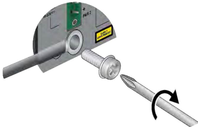
Figure 50. Attaching the Grounding Wire to the Switch
