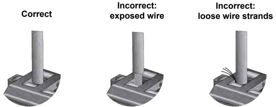
Figure 66. Verifying the DC Power Wire Installation
