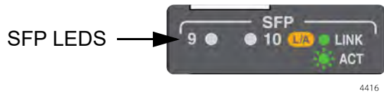
Figure 11. IS230-10GP SFP LEDs: Ports 9 and 10
