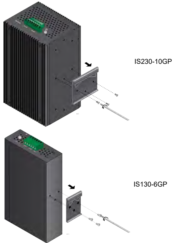
Figure 24. Remove Din Rail Mounting Bracket
