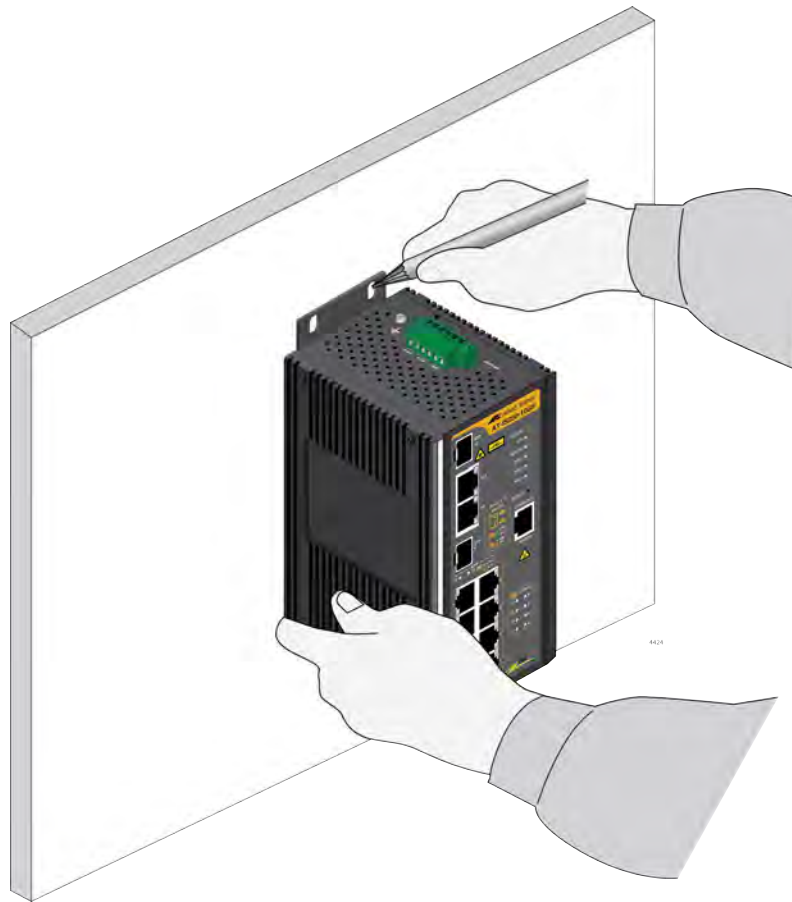
Figure 26. Mark Wall Bracket Hole Locations
