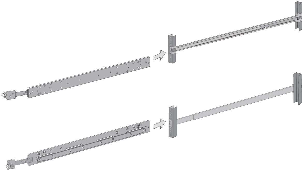
Figure 16. Testing the Inner Rails with the Extension Brackets
