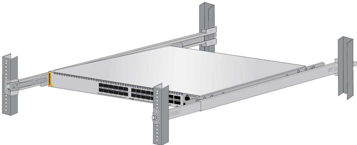
Figure 8. Example of a Switch Recessed in an Equipment Rack
