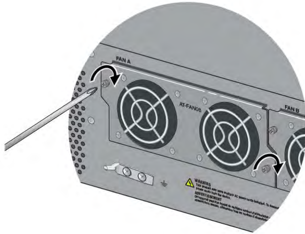
Figure 102. Tightening the Two Captive Screws on the FAN08 Module
