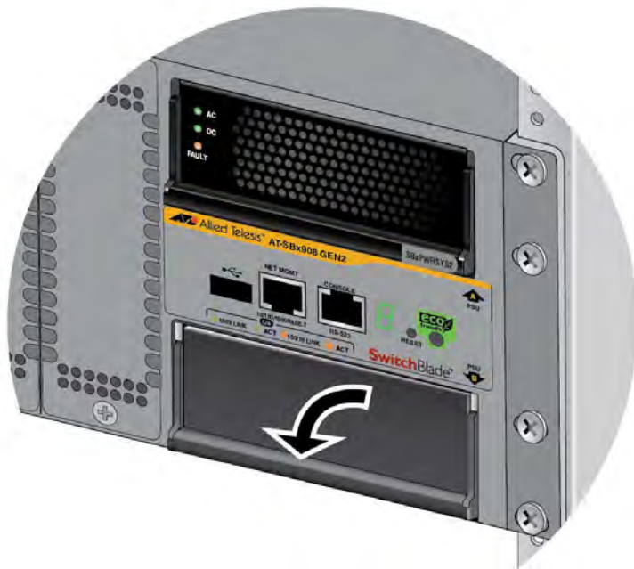
Figure 40. Lowering the Locking Handle on the Power Supply Slot Panel
