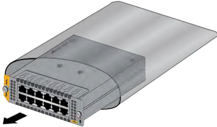
Figure 42. Removing the XEM3 Module from the Anti-static Bag
