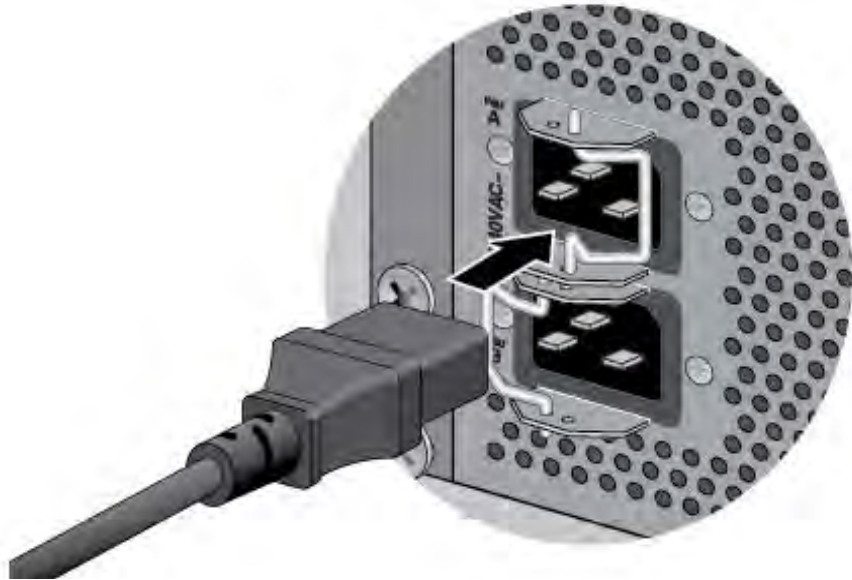
Figure 78. Connecting the AC Power Cord
