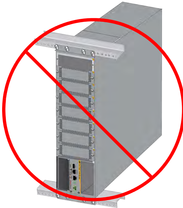
Figure 25. Vertical Installation in Equipment Rack Not Supported
