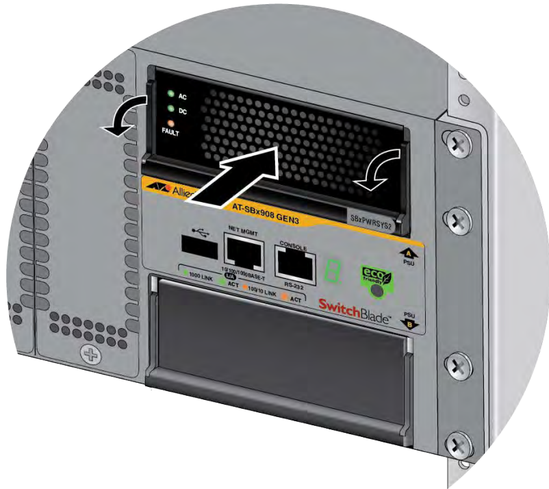
Figure 36. Lowering the Locking Handle on the SBxPWRSYS2 (AC) Power Supply
