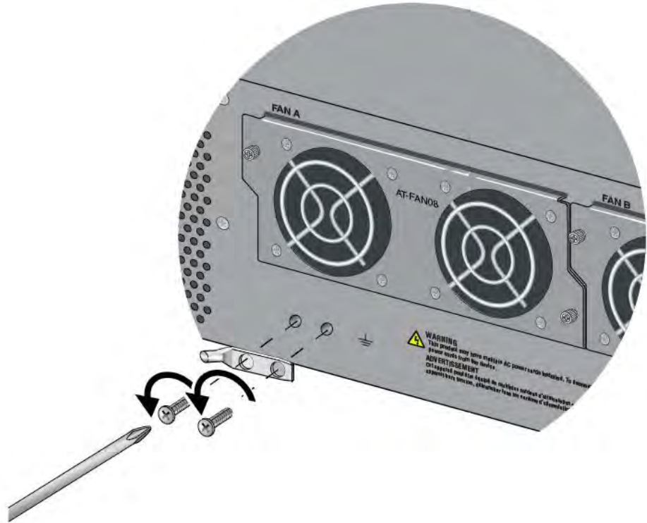
Figure 30. Removing the Grounding Lug from the Switch
