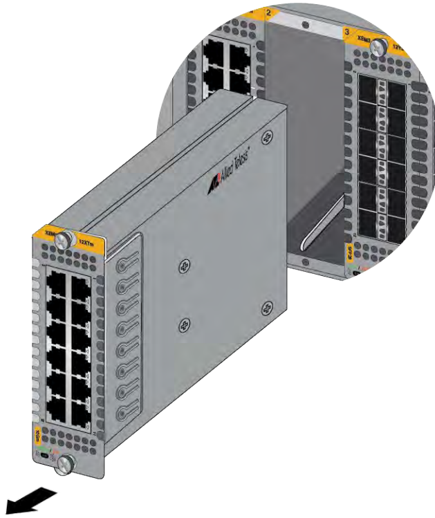
Figure 95. Sliding an Ethernet Module from a Chassis Slot
