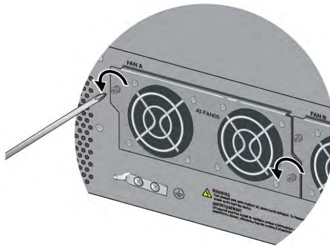
Figure 98. Loosening the Screws on the FAN08 Module
