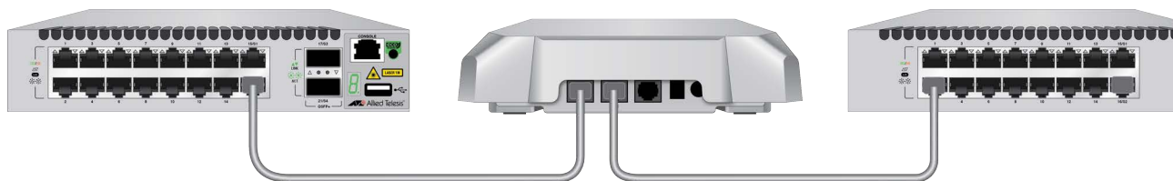
Figure 33. Port2 in Cascade Mode with a Networking Device
