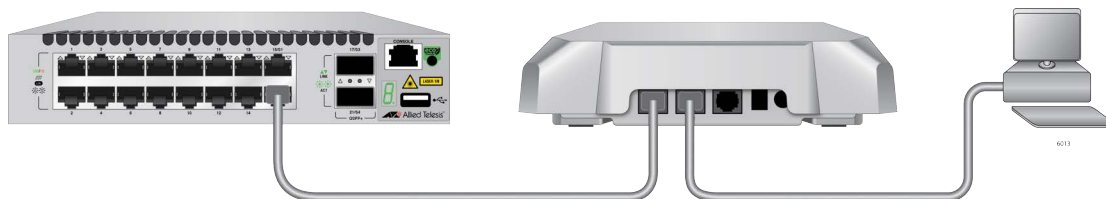
Figure 32. Port2 in Cascade Mode with an End Node
