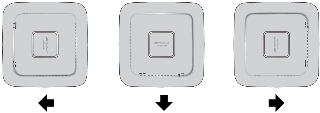
Figure 19. Seating the Access Point on the Mounting Bracket
