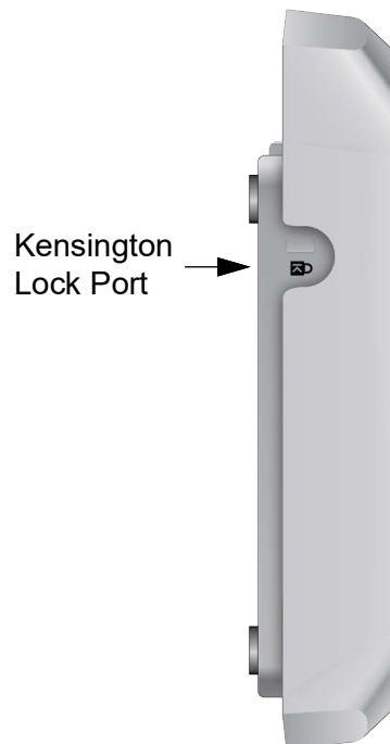
Figure 29. Kensington Lock Port Location
