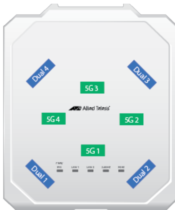
Figure 34. Antenna Axes on the TQ6702 GEN2, TQ6702 GEN2-R, and TQm6702 GEN2 Access Points
