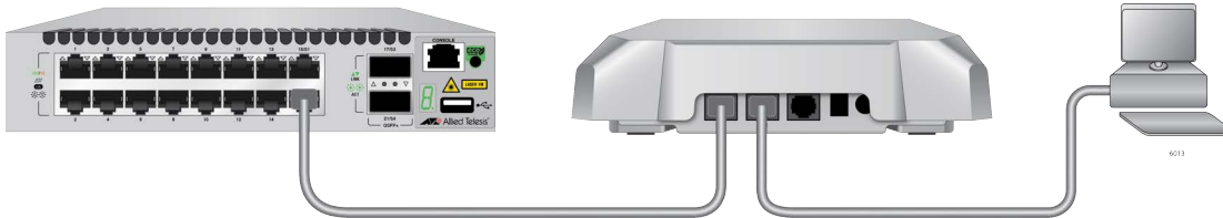
Figure 25. LAN2 Port in Cascade Mode with an End Node
