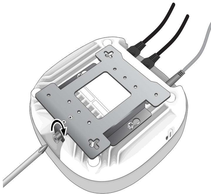
Figure 25. Tightening the Mounting Bracket Thumbscrew
