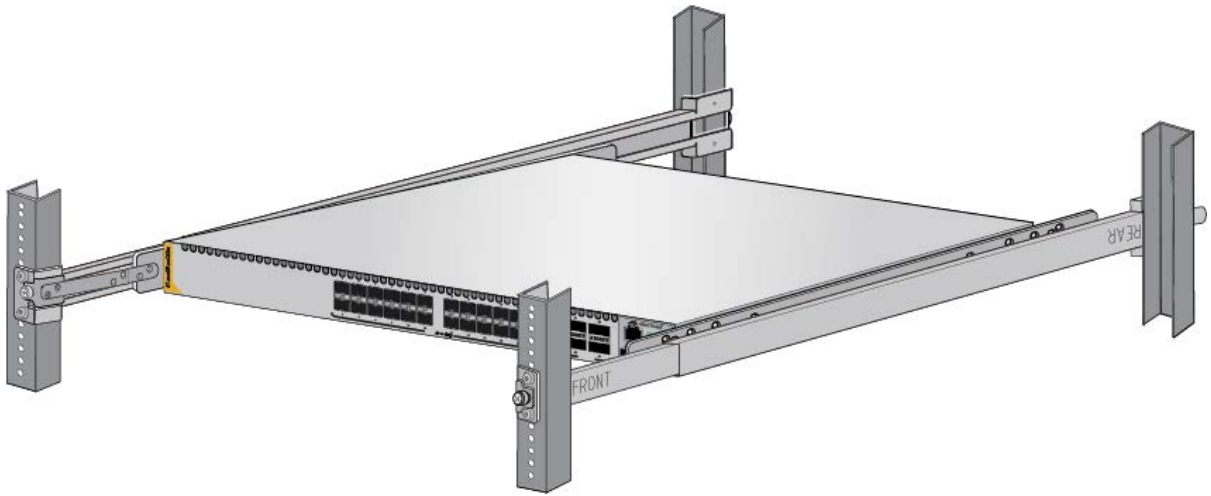
Figure 46. Example of a Switch Recessed in an Equipment Rack
