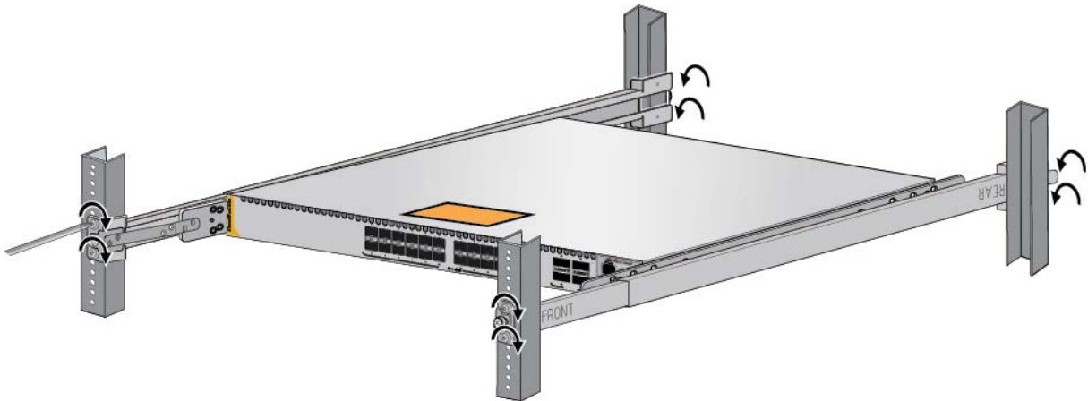
Figure 61. Tightening the Screws on the Outer Rails
