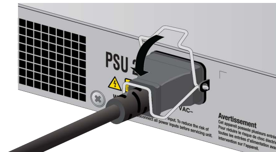
Figure 30. Lowering the Power Cord Retaining Clip
