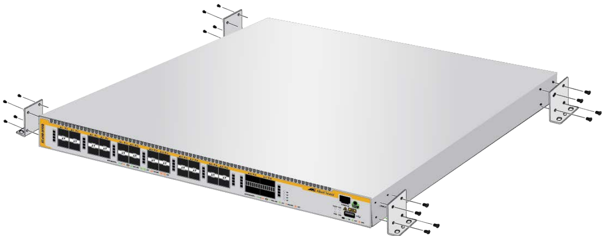
Figure 20. Installing the Brackets to the Switch
