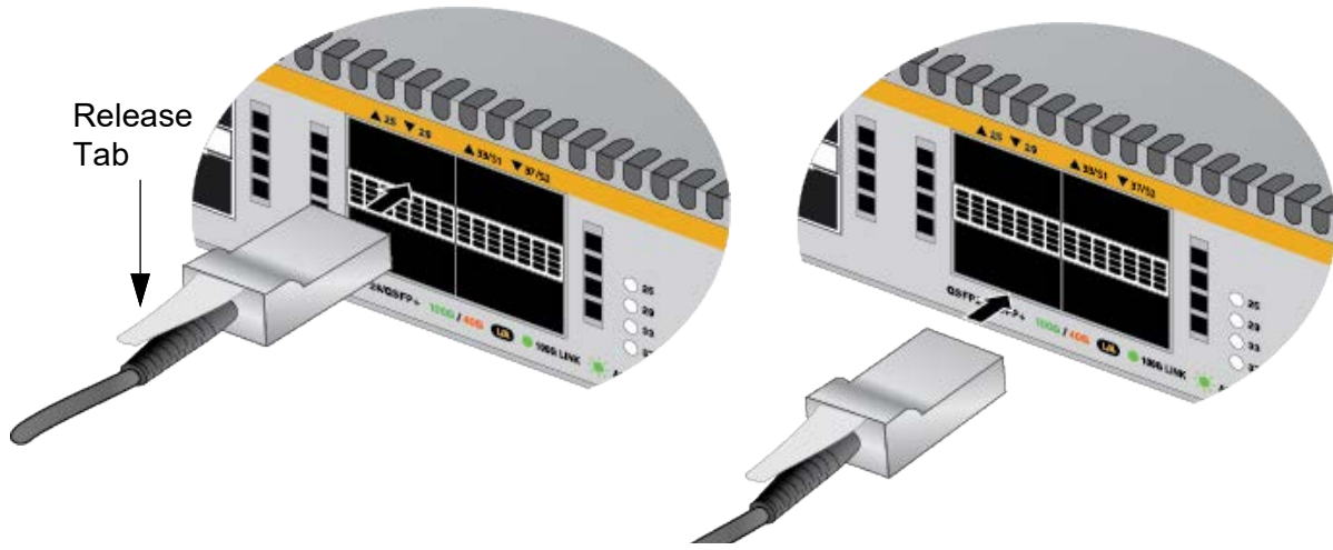
Figure 41. Attaching QSFP28/QSFP+ Cables
