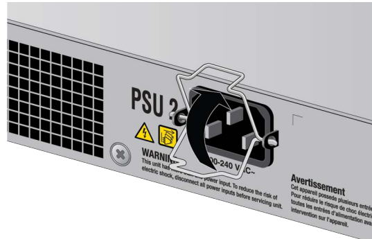
Figure 28. Moving the Power Cord Retaining Clip to the Upper Position
