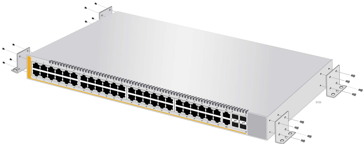
Figure 50. Installing the Brackets to the Switch for Wall Installation
