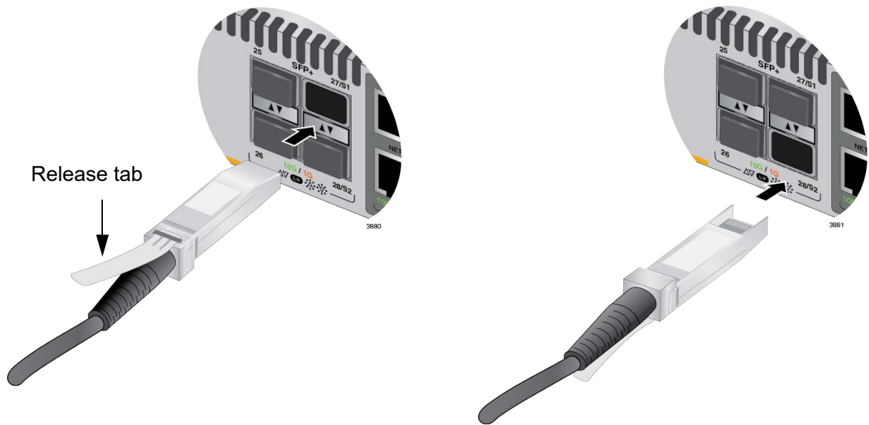
Figure 81. Installing AT-SP10TW Cables
