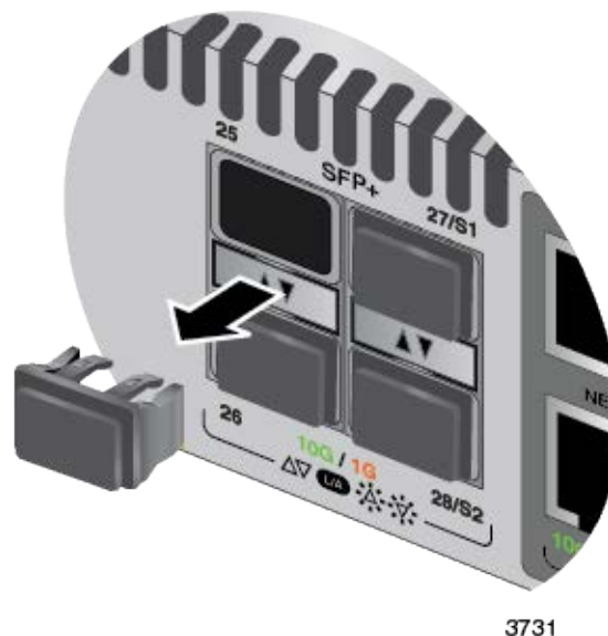
Figure 74. Removing the Dust Plug from an SFP Slot
