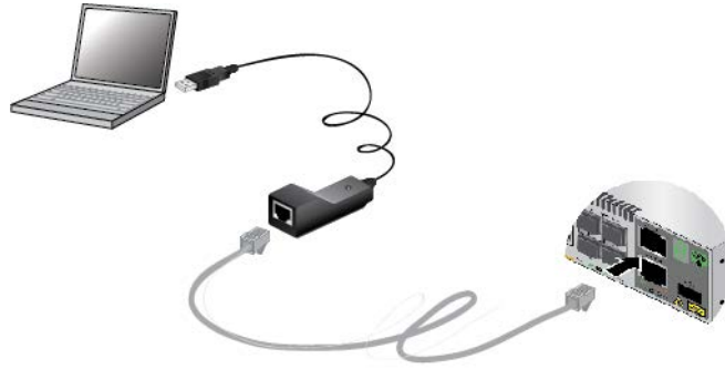
Figure 66. Connecting the VT-Kit3 Management Cable to the Console Port
