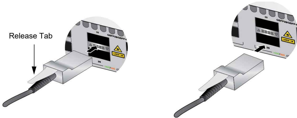
Figure 137. Attaching QSFP28/QSFP+ Cables
