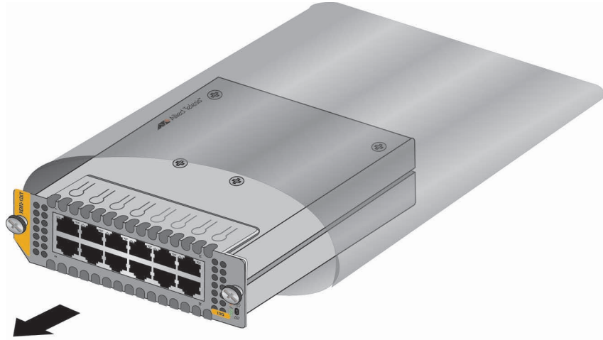
Figure 75. Removing the XEM2 Line Card from the Anti-static Bag
