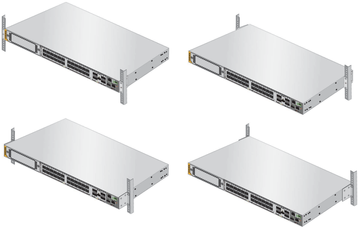
Figure 86. Switch Orientations in an Equipment Rack
