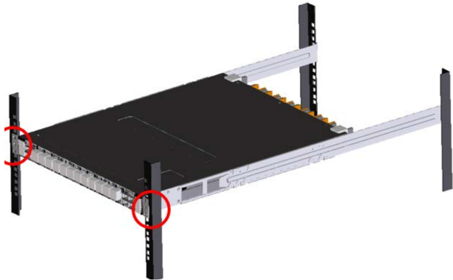
Figure 19. Switch Installed in Four-posts Rack Rail
