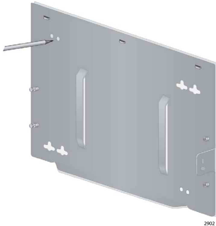
Figure 17. Marking the Locations of the Bottom Panel Holes on the Wall or Ceiling
