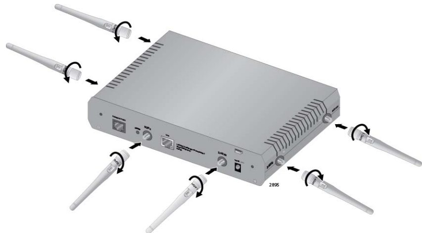
Figure 8. Installing the Antenna
