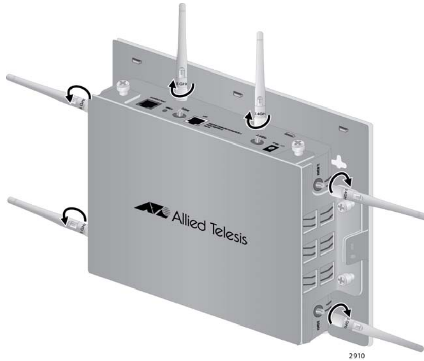
Figure 24. Installing the Antennas
