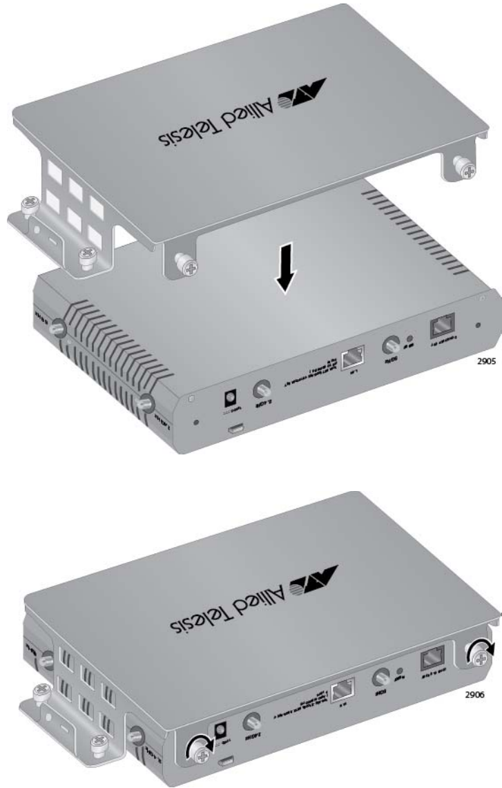
Figure 21. Attaching the Top Panel to the Access Point
