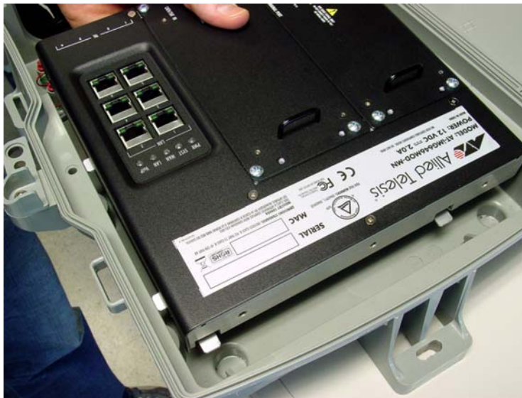
Figure 4. Sliding the gateway into the Enclosure (Tabs into the Notches)
