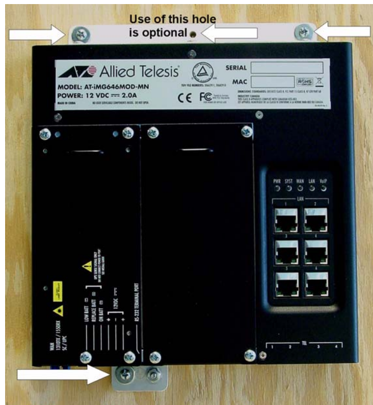
Figure 16. Securing the Gateway to the Mounting Surface
